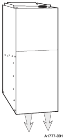
Figure 3: Floor base and ductwork installation - downflow
